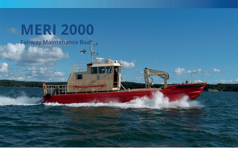
Meri 2000 class fairway maintenance boat is a partially covered, aluminum-hulled boat. It's a traditional fairway station working boat capable of carrying out versatile assignments.
